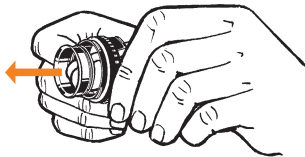
Push the Filling Chamber Cylinder upwards out of the Filling Chamber Housing
